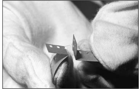
Perforation damage to 8mm film can be repaired with presstape. Because of the small scale, 8mm and Super 8mm films are difficult to repair.
