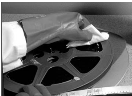
Then gently wipe mold from the film roll with the cloth. For more on cleaning, see 3.6.
