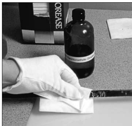
To clean mold from film, gently run the film through a cloth dampened with film cleaner.
