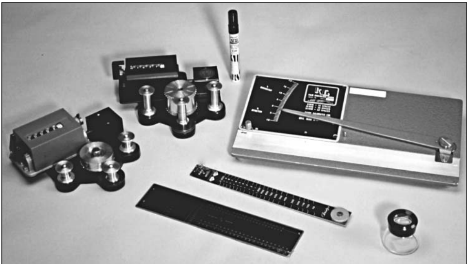
Film measuring equipment (clockwise from left): 16mm footage counter, 35mm footage counter, marking pen, shrinkage gauge, loupe, and film rulers.
