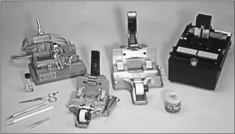
Film repair equipment for every budget (from left): Film cement, 16mm cement splicer, 16mm tape splicer, 35mm tape splicer, repair tape, and 16mm/35mm ultrasonic splicer. Also shown (bottom left): Scissors, X-acto knife, marker, and tweezers.
