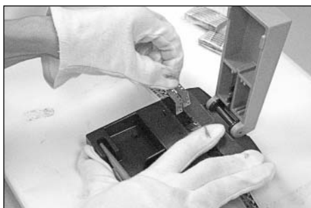
Making a splice using presstape.
